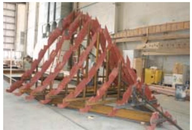
While the keel and stringers are being laminated, the fabrication of the 90-foot hull jig is underway. The jig was shipped to ACY in pieces from the Edison Chouest Offshore shipyard in Louisiana where it was cut out of steel with computerized plasma cutters, ensuring absolute accuracy.
