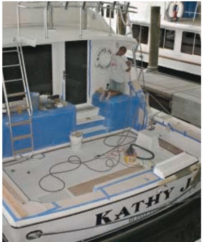
ACY is installing a new teal cockpit sole on the **KATHY JO**, a 60' **Bertram**. The vessel will also receive a complete bottom job and minor gel coat repairs.
