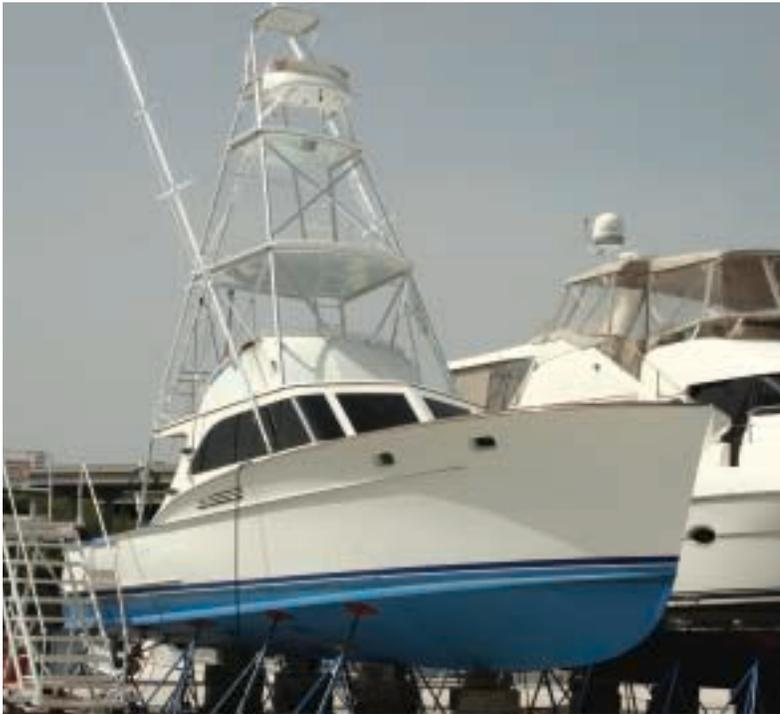
Aptly named, since it was the 20th vessel built by **Rybovich Yachts** in 1955, **TWENTY**, a 43-footer, is visiting ACY for a variety of upgrades. ACY is installing new engine controls and steering, as well as new mufflers, running gear and shafts. The drive line will also be re-targeted. Interior modifications include new carpet, wall covering and headliner. Topping off the project is a new custom tower by BAT.
