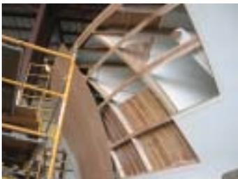
Upon arrival at ACY, the temporary repair was cut away and all damaged wood was completely removed. Once the structural elements were permanently repaired, the hull and deck were re-fitted, then prepared for glassing and fairing to bring back the original integrity.
