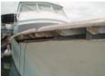
ACY's primary tournament vessel, the 65' **FREEDOM** suffered major hull damage in Brazil after being battered by a sailboat that broke loose during a severe squall. Immediately after the accident, the crew cut away as much damaged wood as possible.
