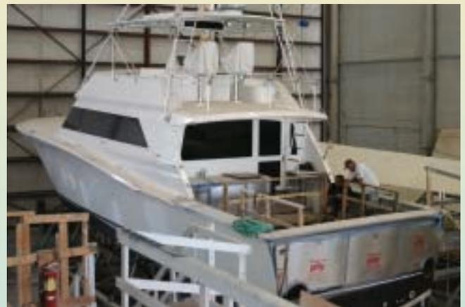
*SALT SHAKER, a 65' Jim Smith, is being prepared for a fuel tank replacement.*
