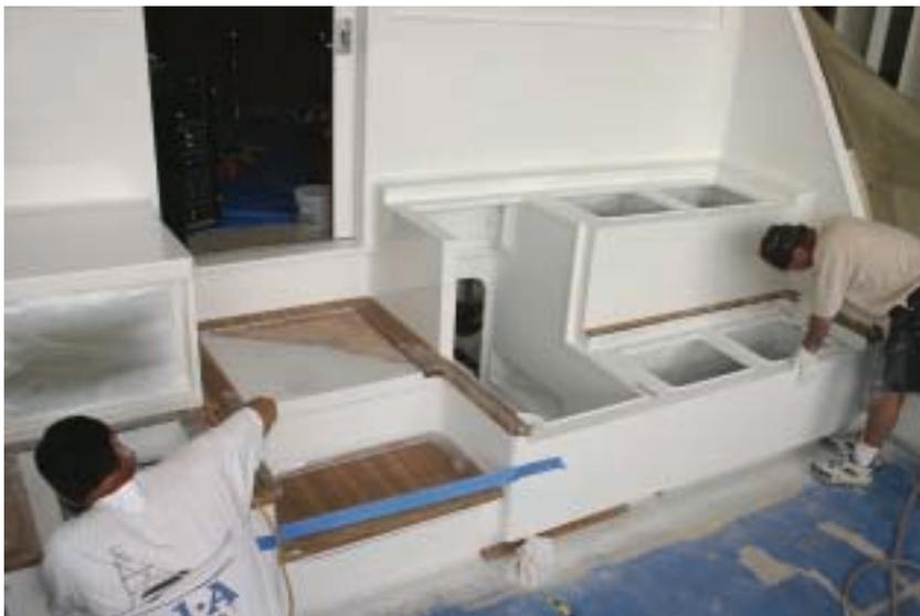
The ROOKIE IV, a 63' Monterey, was built in 1985 with a traditional cockpit configuration. Driven by the owner's desire, ACY created a custom mezzanine to increase refrigeration and storage capacities and give the vessel a more modern appearance. The unique refrigeration cabinets feature SOR® vacuum-bag insulation, taking up half as much space as traditional insulation.
