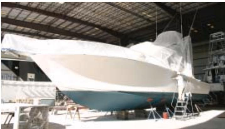
*YOU NEVER KNOW, a 44' Viking, is being prepped for a complete repaint. The vessel will also receive a new teak cockpit and covering boards.*
