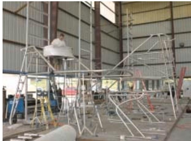
At left, a low profile tower is under construction for **POP-A-TOP**, a 42' **Tiara**. On the right is a full tower for a **Cabo 35**.
