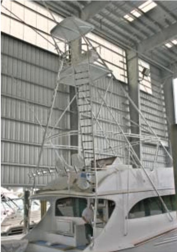
The full tower on the **BLANK CHECK**, a new 68' **Weaver**, awaits installation of the hard top. This tower features every option available, including custom-molded tops, a drop-down radio box, built-in teaser reels and LED lights.
