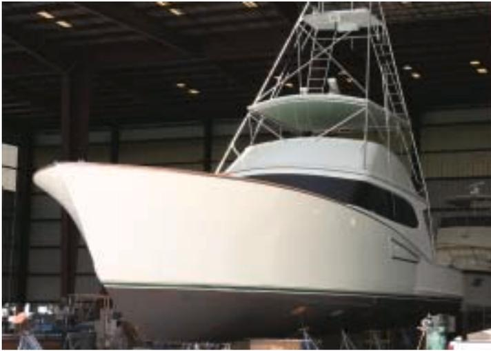
The NUCO2, a 65' **Willis** custom sportfisherman, is visiting ACY for a complete bottom job, as well as splash rail damage repairs and minor paint touch-ups. ACY will also fabricate and install a new sea chest.
