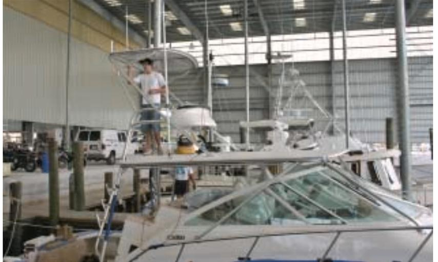
BAT is completing the low-profile tower with a custom molded hard top on the **RED HERRING**, a **Cabo 40**, in preparation for the vessel's delivery to a customer in Spain.
