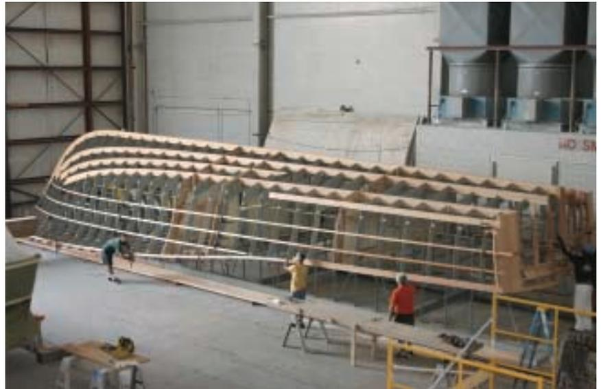
The keel, stringers and structural bulkheads are all in place on the new FREEDOM 68. The transom is now being framed, and the shear and chine are being established with the application of longitudinal battens.
